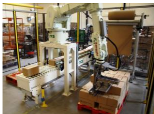
Kawasaki FD050N at Kroes Bakery Dozen, trays met snacks palletiseren
